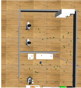
Fig. 12. World Robot Summit arena with the proposed topological graph representation
