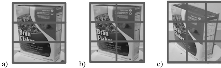
Fig. 1. Example of the sections created to obtain visual features (images from [23]). a) Three windows with size n = 74 , m = 224 ; b) Six windows with size n = 74 , m = 112 ; c) Nine windows with size n = 74 , m = 74
