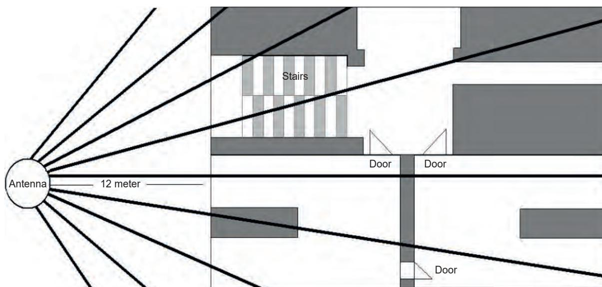
■ **Fig. 23.** The scheme of the experimental site. The transmitter antenna is denoted by circle and located outside the building at the range of 12 m from the front wall of the building. Each line presents the radio path in azimuth domain where the angle is changed from 30 to 150 degrees
