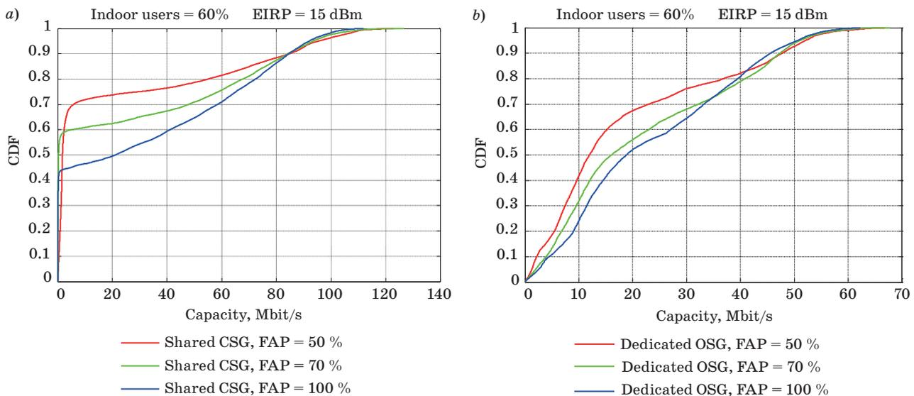
■ **Fig. 20.** CDF of signal capacity for shared CSG (*a*) and dedicated OSG (*b*) for different FAPs densities, of 50, 70, and 100 %, for indoor users using FAP of 60 % from the total number of users in area of service
