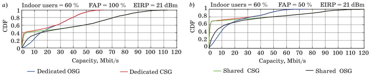
■ **Fig. 19.** Distribution of signal data capacity for four network configurations for different FAP's distribution: 100 % (*a*) and 50 % (*b*). The effective irradiated power is 21 dBm; the number of indoor users is 60 % from all subscribers in the tested area
