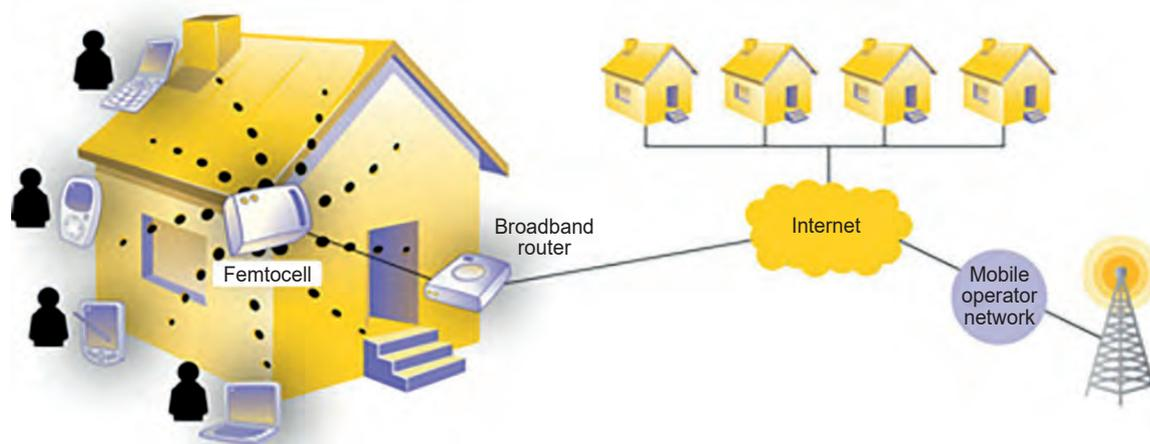
■ Fig. 17. Schematic presentation of Femtocell-WiFi-WiMAX configuration
